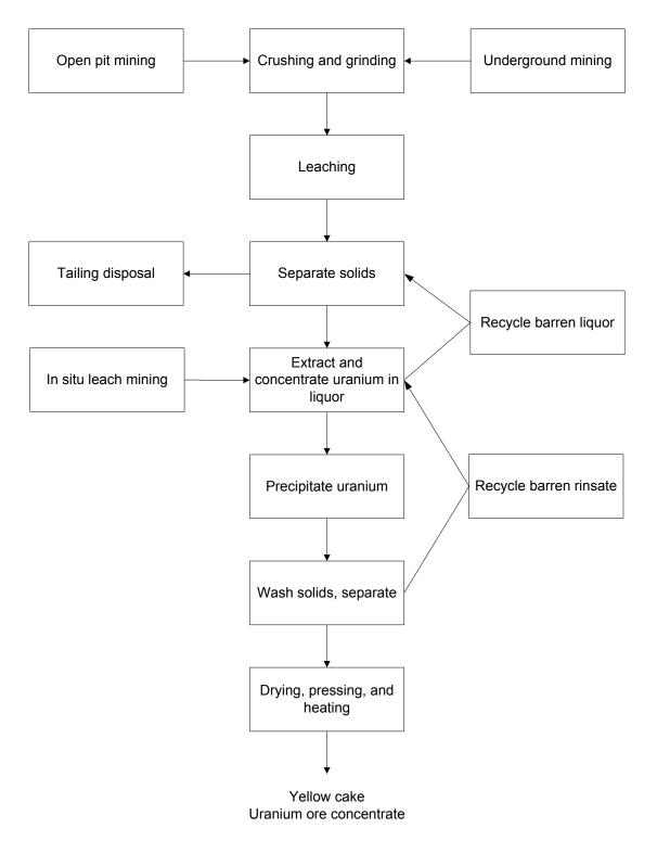
Figure 5-1. Uranium Ore Processing
